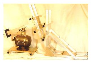
**Figure 14 Separation Reliability Fixture**
