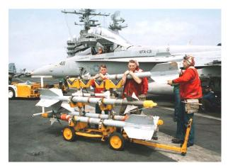
Figure 4 integrating an air-to-air missile to an F-18 aircraft
