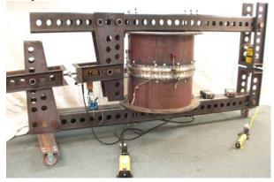
Figure 12 Strength test fixture
