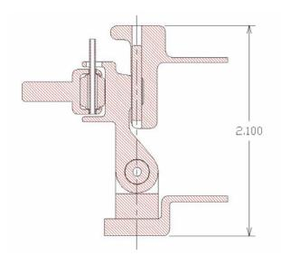
Figure 10 Cross-section of Motorized Lightband. Dimensions are in inches.
