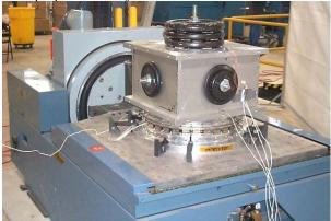
Figure 13 Vibration test fixture, Lightband and electro-dynamic exciter
