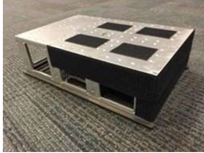
Figure 32. Assembled CubeSat Chassis with Hook and Loop Tape
