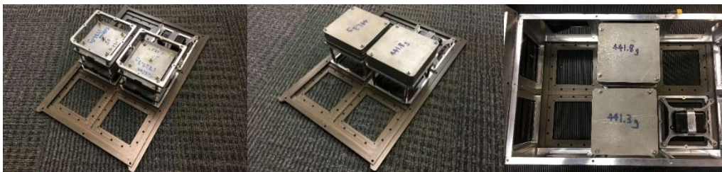
Figures 21, 22, 23. Centered COM Mass Stack Setup (left), Top-Heavy COM Mass Stack Setup (center), Mass Stacks in Chassis (right). Note CubeSat chassis top is removed for easier visualization.
