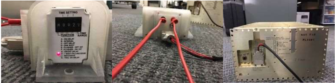
Figures 36, 37, and 38. Trigger Settings (left), Trigger connections (Center), Trigger CSD Connection (right)
