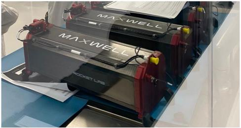
O PLANET SUPERDOVES BEING INTEGRATED WITH ROCKET LAB MAXWELL DISPENSERS
