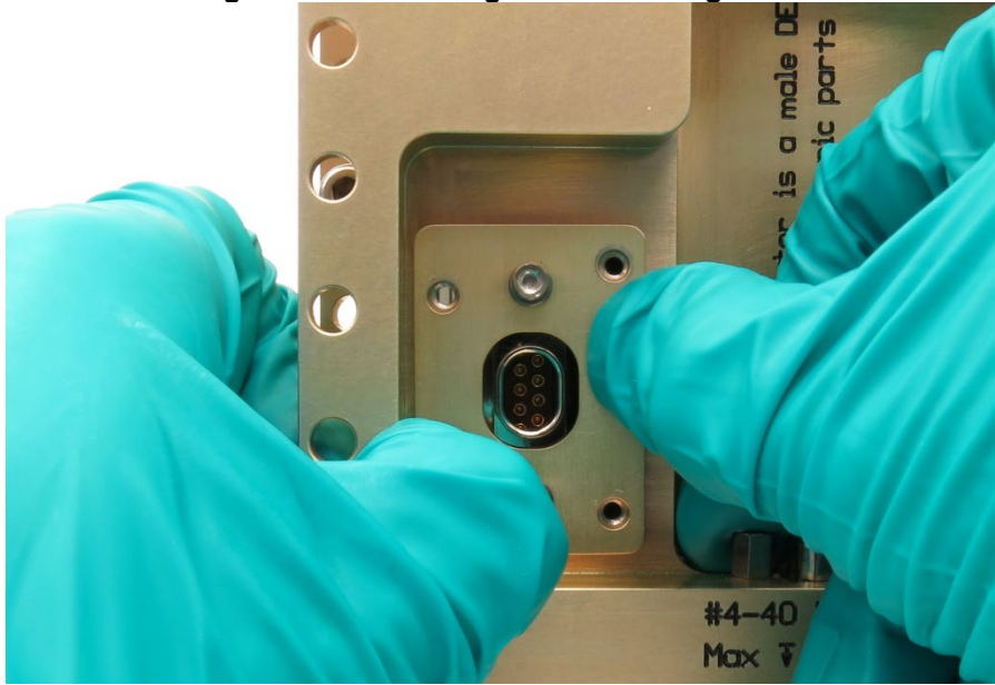
Figure 8-16: Securing Connector to Plate and Plate to CSD
