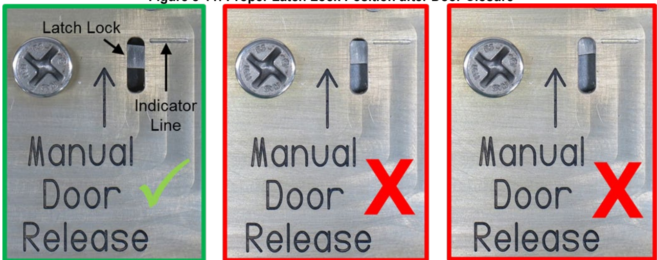
Figure 8-11: Proper Latch Lock Position after Door Closure
